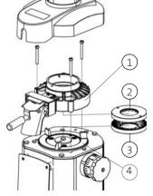
9.2.1.2Removing the grinding disc in the stationary flange, without screws
