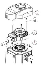
9. Replace the bean hopper as described in section 9.1.1 "Removing / Replacing the hopper".
